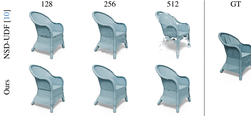
Figure A.1: Meshing at different resolutions, additional examples. While NSD-UDF [10] retrieves most of the surface well at a low resolution, it struggles at higher ones. In contrast, our method, recovers the surface well at all resolutions. We use Marching Cubes with both methods.
